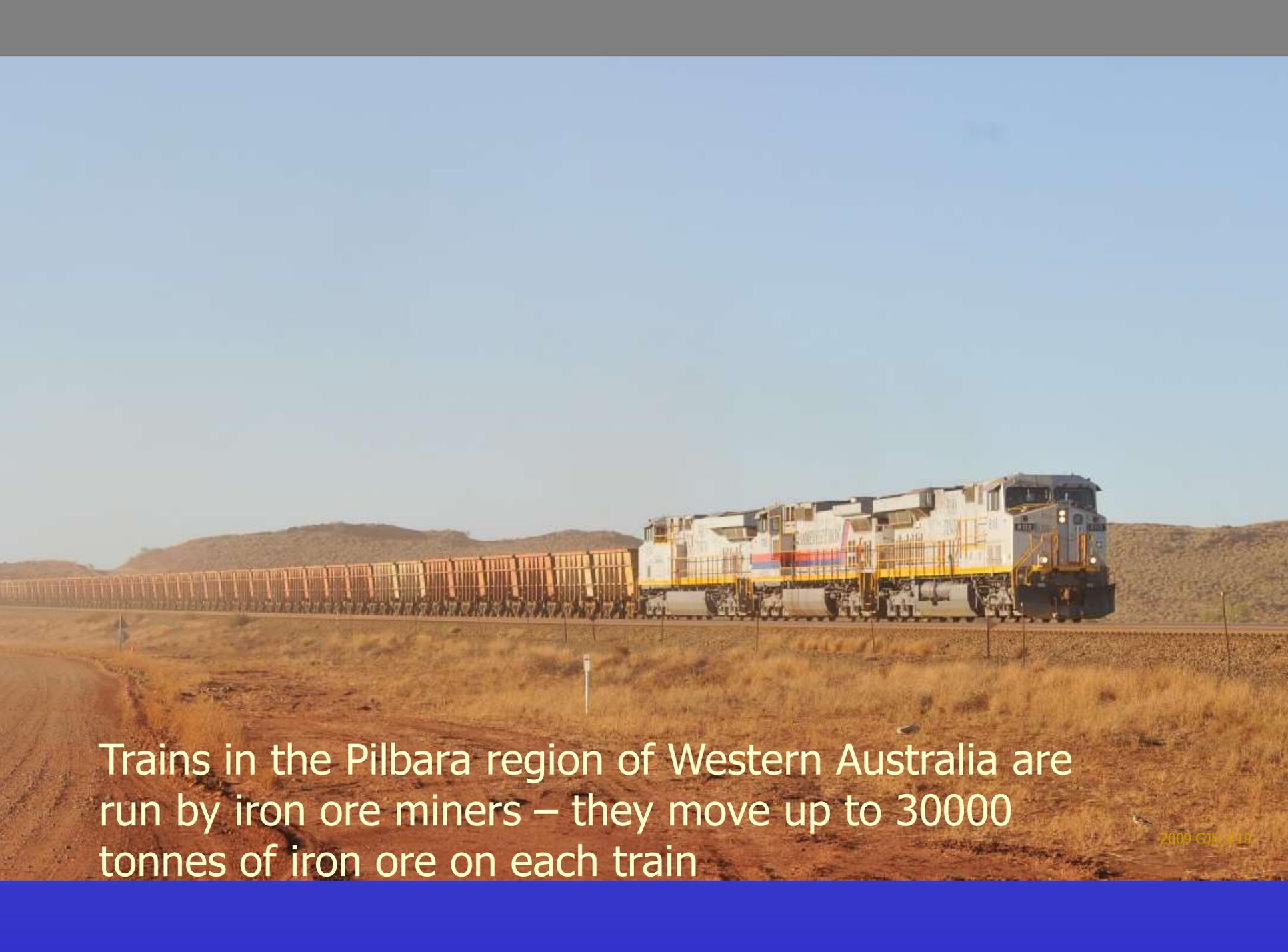
Trains in the Pilbara region of Western Australia are run by iron ore miners – they move up to 30000 tonnes of iron ore on each train
